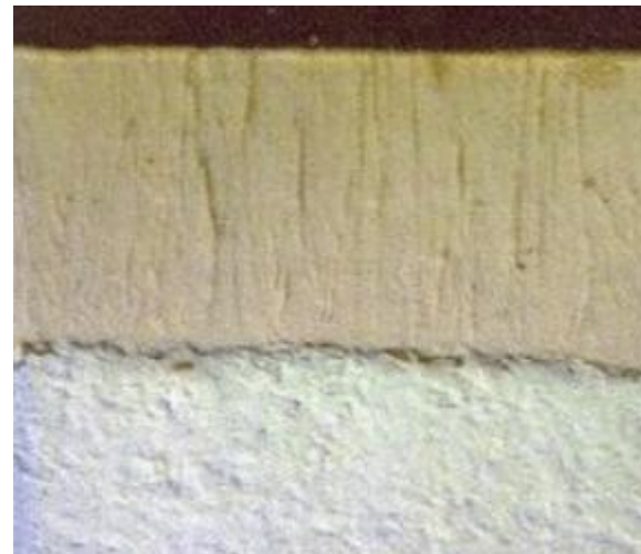
Cross section of EL Nickel Boron after 380 hours of salt spray corrosion test
